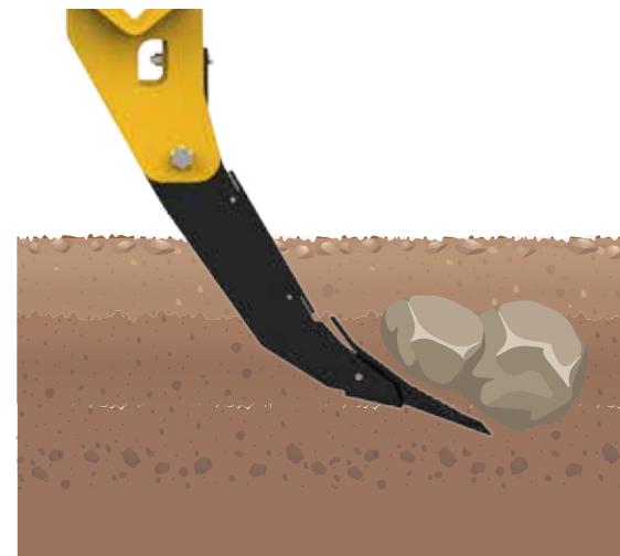
MECHANICAL SHEAR BOLT Safety solution introduced by Alpego, a mechanical safety shear bolt fitted on every shank; if the shank hits an obstacle, the bolt shears, protecting the machine structure.
