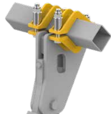
SHANK MOUNTING Clamps are diagonally fitted to reduce stresses on bolts, minimising the number of bolt failures. Standard on models: K-DYNO / K-EVO / K-FORCE / K-EXTREME
