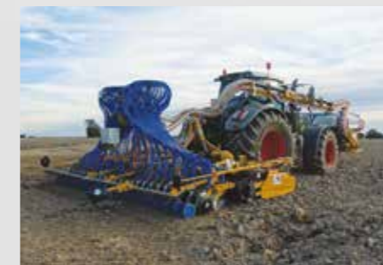
Fertidrill ASMAX BITUBE with power harrow Alpego
