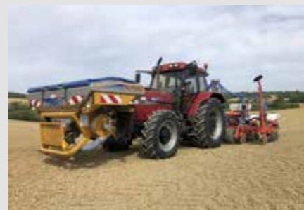
Fertidrill ASPRO with precision seed-drill
