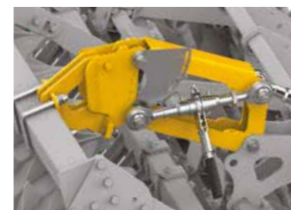
Quick release system of the seeding bar from the power harrow.
