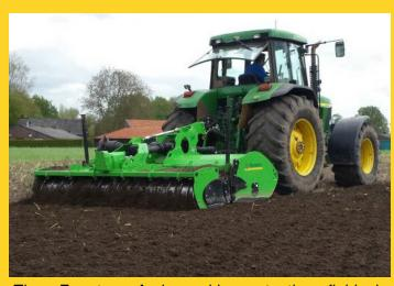
The Farmtec Agri working at the field in combination with harrow-roller at a sandy soil.
