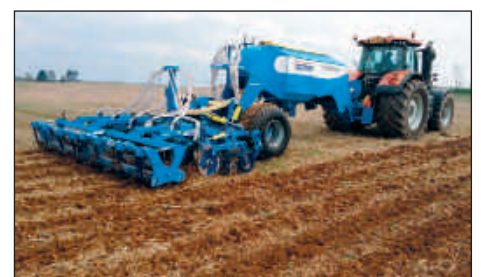
Mounted cultivator for strip-till soil cultivation.
