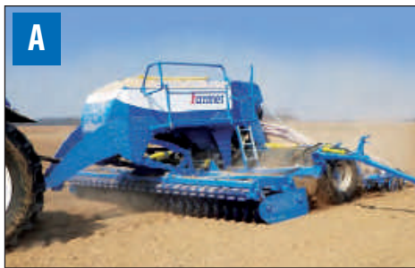
Sowing of cereals into narrow lines with possibility of fertilization under the heel.
