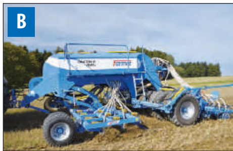
Sowing of rape with deep loosening and fertilizer application.
