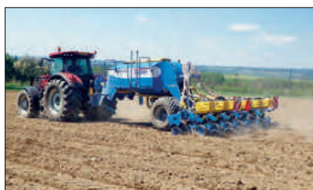
Mounted seed drill for sowing wide-row crops.
