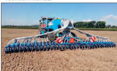
Wide seeding bar for sowing close-drilled crops.
