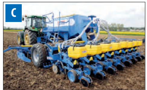
Precision sowing of corn and fertilizer application.
