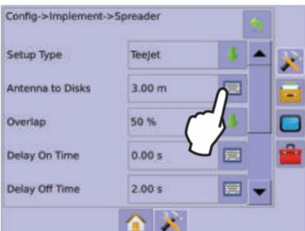
Enter the distance between the antenna and the centre of the spreader.
