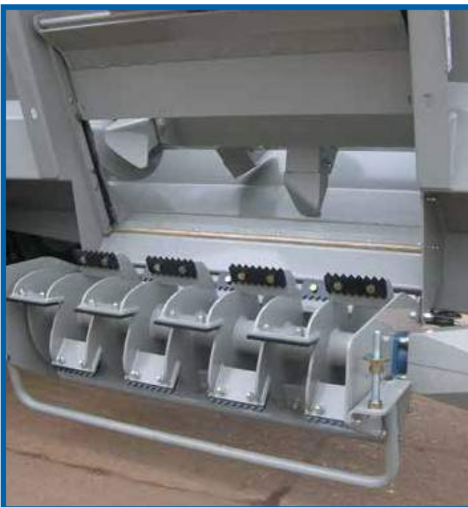
Discharge rotor can be hydraulically lowered to allow access
