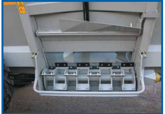
1.4m wide rotor with Hardox bolt on wear plates
