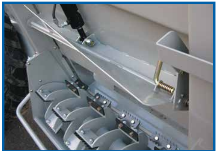
Adjustable slurry deflector controls discharge height
