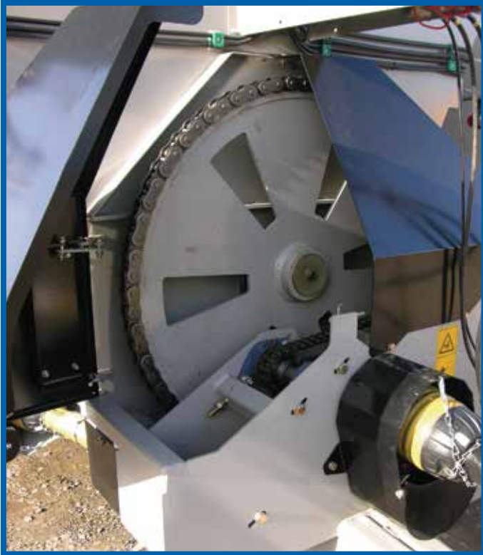
Simple high power chain drive with reverse
