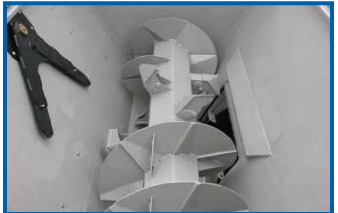
Hydraulically operated anti bridging arm keeps material moving to the door
