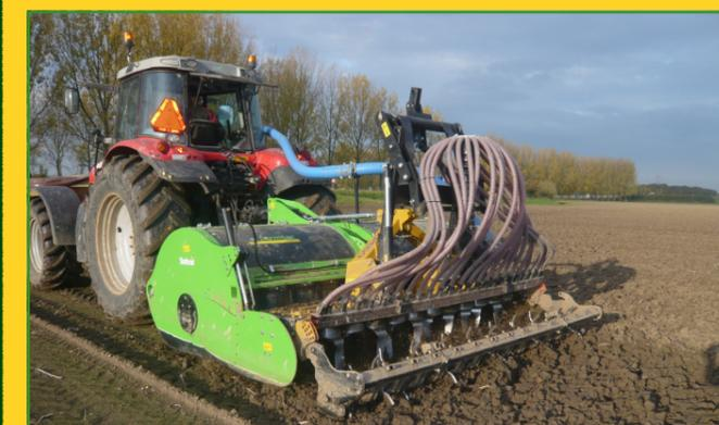
The Rotar digging machine in combination with a Alpego power harrow is a excellent tool for digging and drilling in one pass. The advantage is that you do not drive one the soil before drilling.
