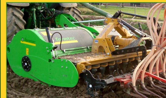
The Rotar digging machine is equipped with center drive (no chains in the machine!). With a direct PTO drive to the Alpego power harrow . The Alpego power harrow is integrated at the digging machine.
