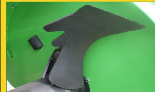
The Rotar Farmtec digging machine is specifically designed for the heavier soil. The special shape of the blade with a "upside down / outbreak" operation. The ground is broken and the structure of the soil guaranteed. By maintaining or improving the structure, improve soil permeability and the capillary effect is improved.
