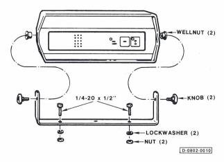
Step 1. Refer to the above illustration and using the U-shaped mounting bracket as a template, mark the location of the two outside bracket mounting holes.
