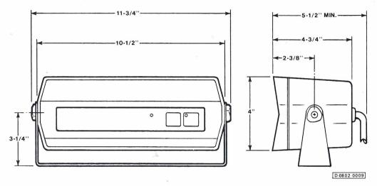
Refer to the above illustration and select a location (on hood, fender or within cab) where the console can be easily viewed and operated. The console can be mounted two ways: Procedure 1 uses two bolts to secure the mounting bracket and Procedure 2 uses a single bolt to secure the mounting bracket which allows the console to swivel.
