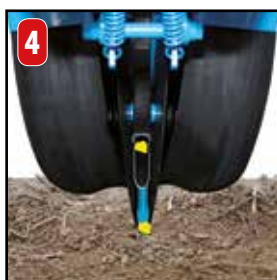
4 The curved seed chute tube has been specially designed to accompany the seeds gently into the ground and with a perfect accuracy.
