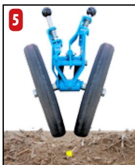
5 The adjustable open press wheel unit*, made up of 2 V-wheels, closes the furrow around the seed for optimal seed germination.
