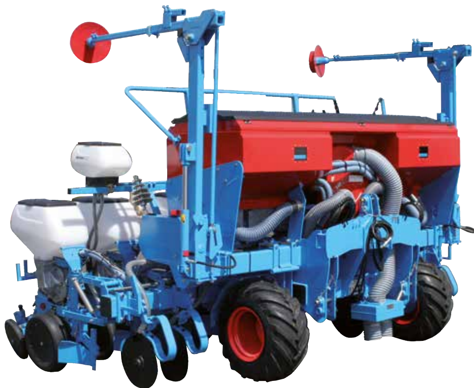
6-row Monoblock2 Comfort planter with fertilizer 680 L and Microsem
