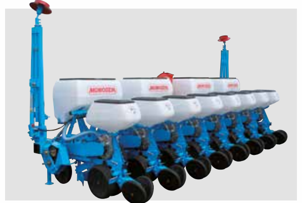
8-row rigid Double bar planter (70 cm inter row spacing)
