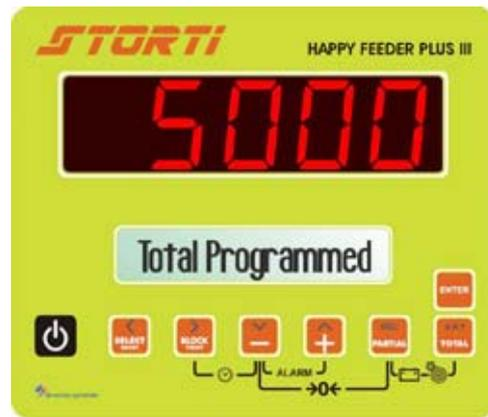
7 At the end of the setting, with the printer connected, when the message TOTAL PROGRAMMED is displayed, it is possible to print the recipe/unloading program by pressing the BLOCK PRINT key.
