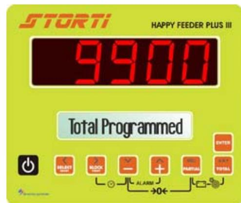
b) If the program/unloading point is programmed per TOTALS, i.e. the Cows' number is = 0, the TOTAL PROGRAMMED appears. It is possible to change this value by pressing the MINUS and PLUS keys.
