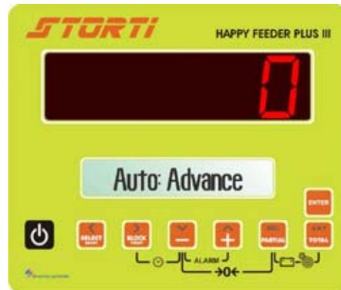
**8 Press at the same time the PARTIAL and TOTAL keys and the indicator will display -PS- PASSWORD-.**
