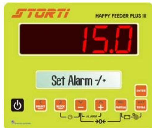
c) Confirm the set weight by pressing the PARTIAL key and go on with the load/upload phase. The weight is displayed with a decreasing order, despite the fact it is loading/unloading.
