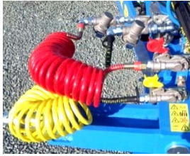
Two-line single-circuit air pressure brakes (a part of standard equipment)
