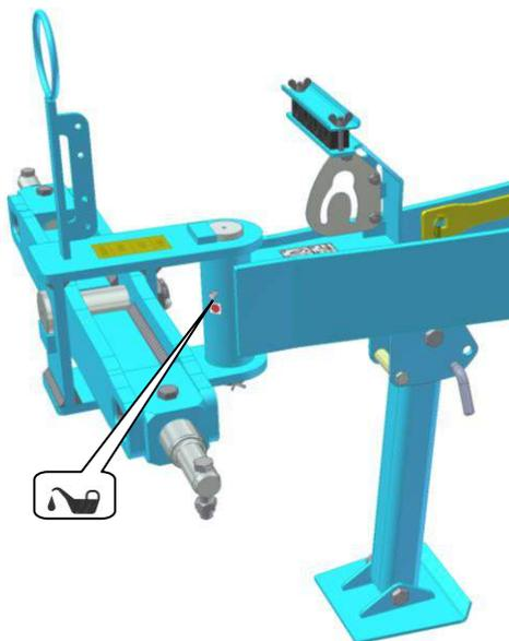
Fig.15- Rollers bearings
