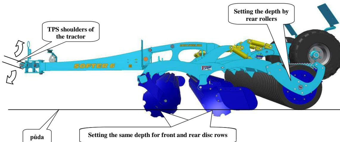
The machine features high stability during operation. However turning of machine to one side may occur with fault adjusted longitudinal plane (particularly in heavy soils). This is removed by modification of tractor arm height as follows:
