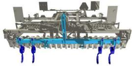
**Track cultivator** – the design of the carried machine does not allow mounting the track cultivator directly to the machine. Therefore, it is possible to attach an additional frame with track cultivators between the tractor and the machine. The frame of the track cultivator is connected to Kompaktomat using a three-point hitch.
