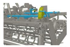
**Hydraulic depth** – controlling the working depth of the shares by the hydraulic circuit from the driver's position
