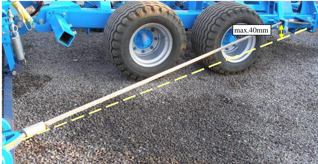
Fig.14 – Prestressing of the tractive rope
