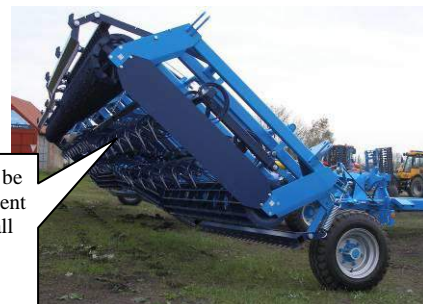
Fig.30 – Working section for ploughshare replacement in the field
