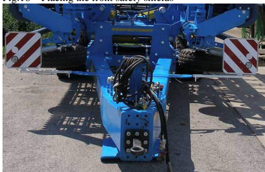
Fig.18 – Placing the front safety shields
