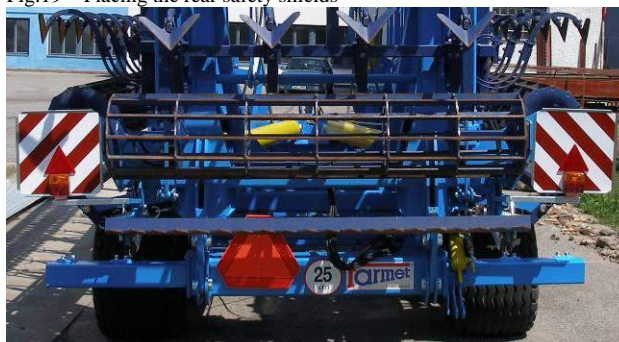
Fig.19 – Placing the rear safety shields
