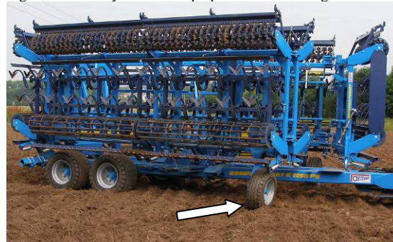
Fig.10 – Auxiliary wheels are prepared for unfolding
