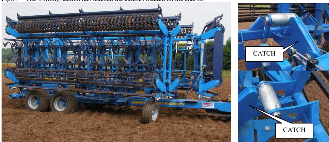
Fig.17 – The working section has reached the catches located on the chassis
