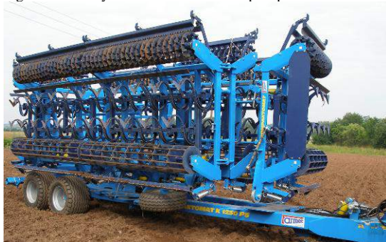
Fig.9 – Auxiliary wheels are in the transport position
