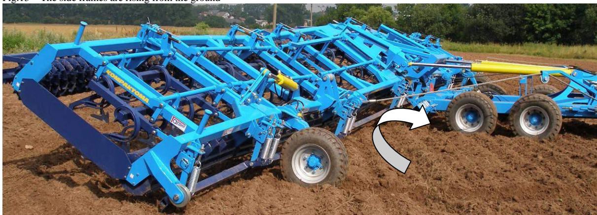
Fig.15 – The side frames are rising from the ground
