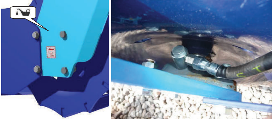
Picture 14 – Lubricating the rear roller bearings
