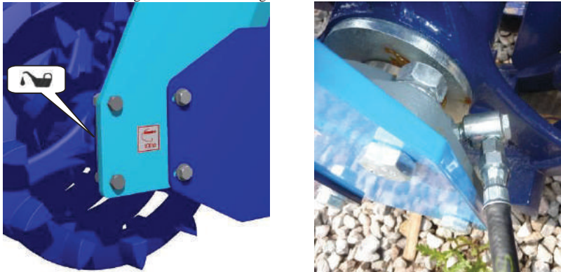
Picture 14 – Lubricating the rear roller bearings
