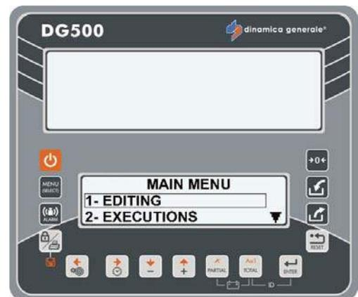
2 Select the component name that has to be set/modified with the PLUS and MINUS keys from Component 1 to 48.
