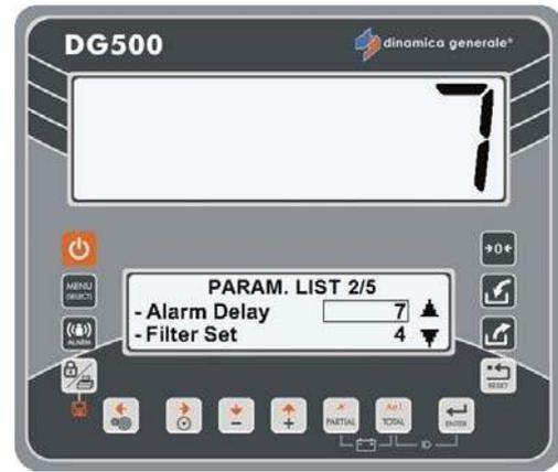
**6 SETTING OF THE FILTER FOR THE WEIGHT STABILIZATION**
