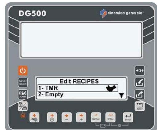
**12** It is always possible to exit from the programming of the Recipe and return back by pressing the RESET key; in this case the message **SAVE CHANGES?** appears.
