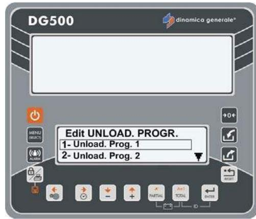
**17** It is always possible to exit from the programming of the Unloading Point and return to PROGRAM UNLOAD by pressing the RESET key; in this case the message SAVE CHANGES? appears.
