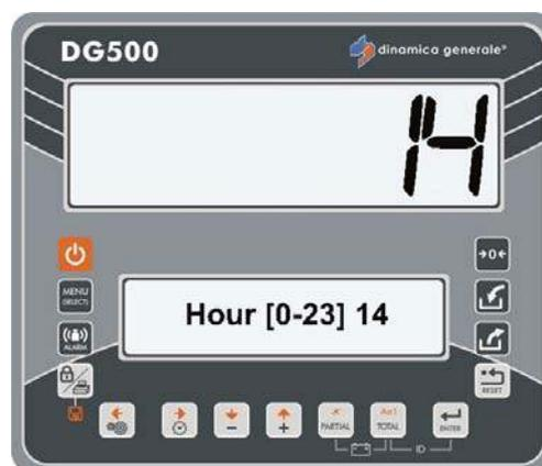
c) Confirm the value with the **ENTER** key (the value will also be seen on the upper display) afterward the indicator will pass on to the next parameters that are:
