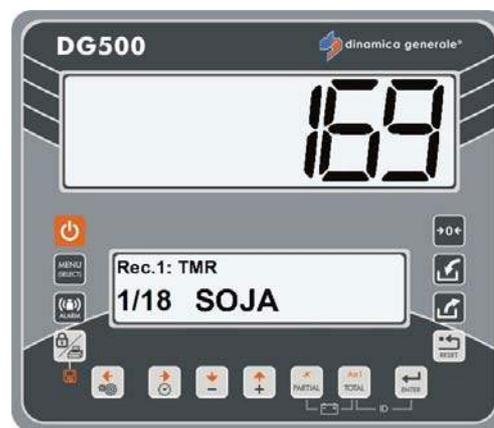
8 The passage from one component to the other can take place by pressing the ENTER key or the PLUS key.
