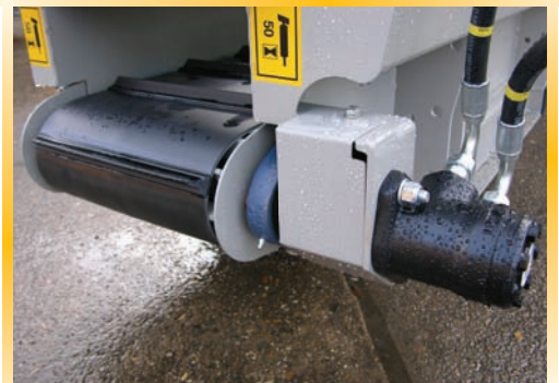
Heavy duty bearings, rollers and ribbed belt
