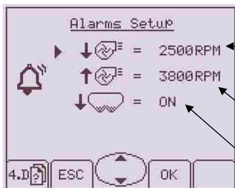
It shows the minimum speed of the seed distribution fan below which the monitor will display the min. RPM alarm
