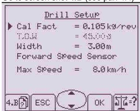
In this screen shot it is possible to manually modify the calibration rate.
