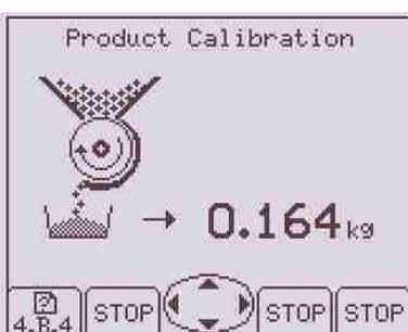
Wait for the metering unit to fill up the container for the calibration test.
