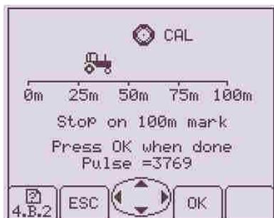
4. Start working with the machine during the test and press the key under the "OK" icon
