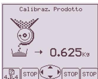
A screen shot like this one will appear and the value of the weight will begin to increase as the seeds drop into the calibration test container
