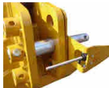
The pin of the micro-switch must always be positioned below the top link of the 3-point hitch.
