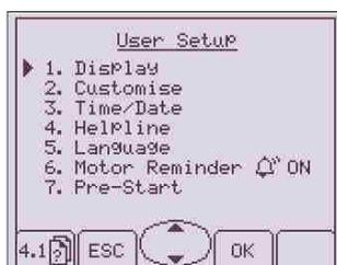
By pressing the middle key in the direction of the arrows as shown in the icon (of the key) the cursor is moved to the various titles of the menu and by pressing the key under the "OK" icon the following screen shots are accessed:
