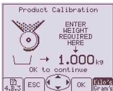
Enter the seed quantity (through the keyboard) which you wish to obtain from the calibration test and press the key under the “OK” icon to confirm the value.
