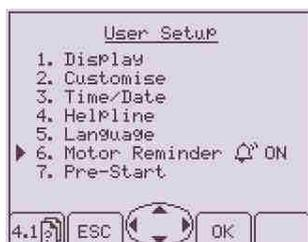
By selecting title **6** “Motor Reminder” you choose to activated an acoustic alarm ON whenever the motor is blocked by lifting the machine.
