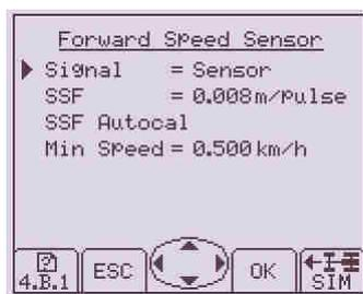
**Signal:** It mentions the device by which the speed is recorded (cannot be modified)
