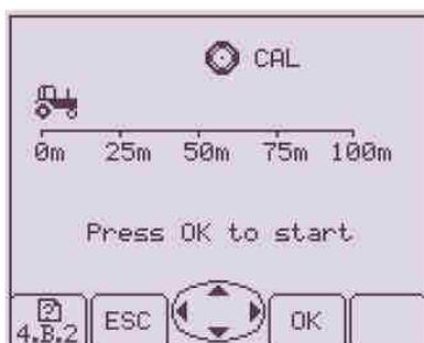
2. Start working with the machine during the test and press the key under the "OK" icon
